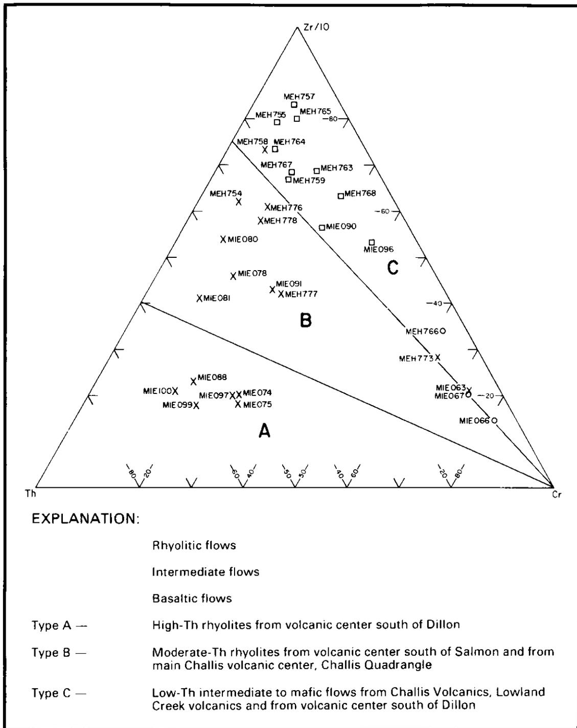
Figure 3. A ternary Zr-Th-Cr discrimination diagram for flow rocks from Dillon and Dubois Quadrangles.
